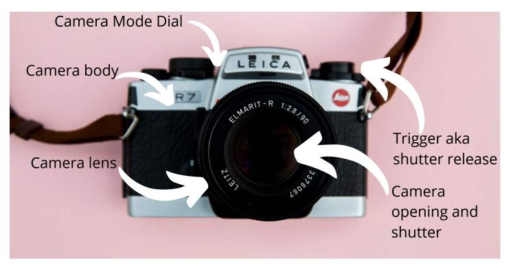
To keep it simple, your camera has a camera body and a camera lens, which attaches to the front of the body. There is an opening of your camera that takes in light and your pictures, and there is a shutter release (or trigger)
